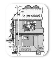
prevent radon gas from entering the home from below the concrete floor and from outside the foundation. DEP-certified radon mitigation contractors may use other methods that may also work in your home. The right system depends on the design of your home and other factors.
