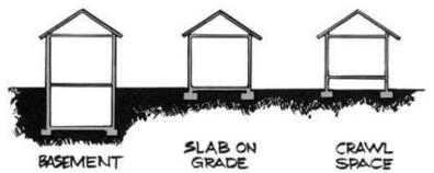
For instance, it is common to have a basement under part of the house and to have a slab-on-grade or crawlspace under the rest of the house. In these situations a combination of radon reduction techniques may be needed to reduce radon levels to below 4 pCi/L. Radon reduction systems can be grouped by house foundation design. Determine your type of foundation design and read about which radon reduction systems may be best for your house.
