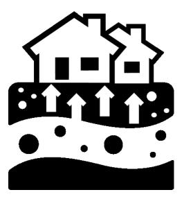
R adon is a naturally occurring radioactive gas produced by the breakdown of uranium in soil, rock, and water. Air pressure inside your home is usually lower than pressure in the soil around your home's foundation. Because of this difference in pressure, your house acts like a vacuum, drawing radon in through foundation cracks and other openings.
